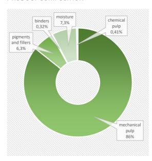
This product contains biomass carbon, equivalent to 1 455 kg of CO2 per tonne of product.
